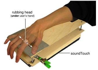
Figure 1. Rubbing interaction implemented using our sound-Touch prototype.
