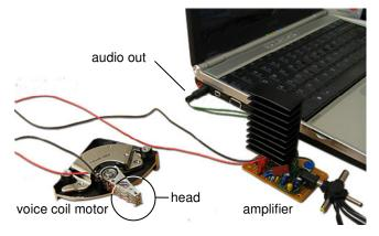
Figure 2. Our *soundTouch* prototype translates sound signals into tactile feedback.
