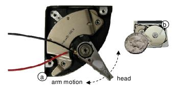
Figure 3. (a) Close-up of the voice coal motor in soundTouch (b) micro drive next to a US quarter.
