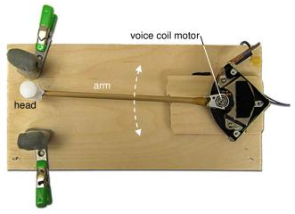
Figure 7. Rubbing prototype (cover removed).
